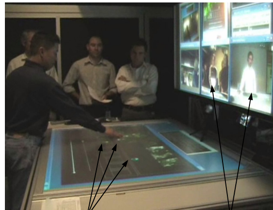
Figure 1. The ViCAT table at one of four sites, sharing a multimodal video editing application on the horizontal screen.
