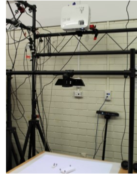
Figure 2: The SAR-TAM tabletop with projector, tabletop and pose Kinets and OptiTrack system (red cameras)
