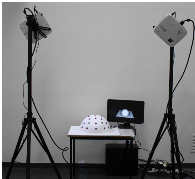
Fig. 2: Hardware setup of the experiment. Two projectors displayed annotations on the dome apparatus.
