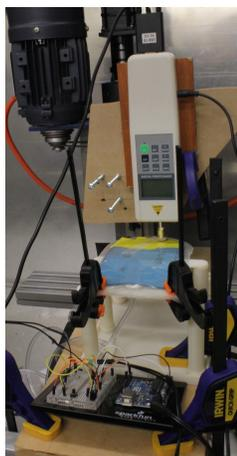
**Figure 3: Experimental setup using our improved wearable bladder attached to a CNC machine.**
