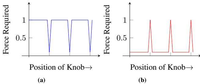
**Figure 1: Slider force configurations. a) Momentary 'clicks' to alert the user towards discrete values. b) 'Detents' at discrete values.**
