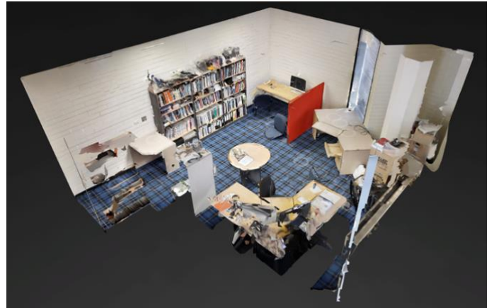
Figure 3: The mesh of the reconstructed office.
