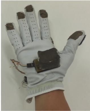
**Figure 1.** The new Passive Deformable Haptic Glove
