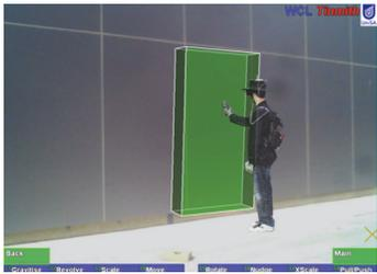
**Figure 4.** Door cut-out model added to the wall, with the user (artificially overlaid) performing the task.
