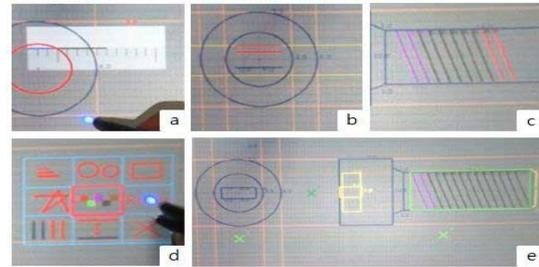
**Figure 1.** (a) Magnifying Glass Tool. (b) Mirroring Tool. (c) Replication tool. (d) Ruler detection. (e) the front and side view of a bolt
