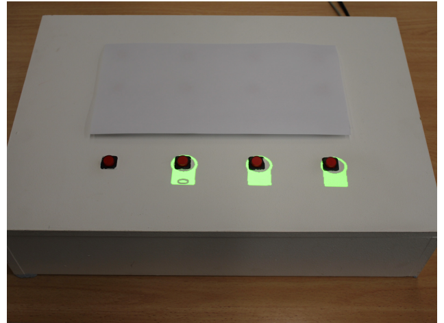
Figure 3: The button box used during the experiment. Three buttons have been highlighted with SAR annotations, with the target shown on the button second from the left.
