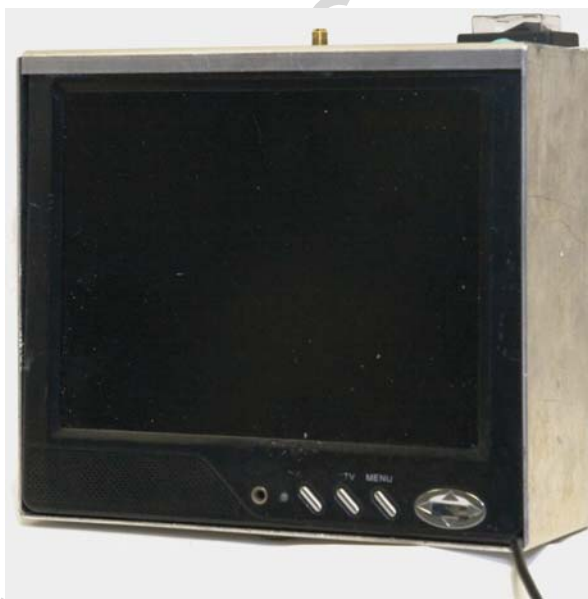
854 Fig. 11.10 External display containing an LCD panel and an integrated battery and wireless video 855 receiver
