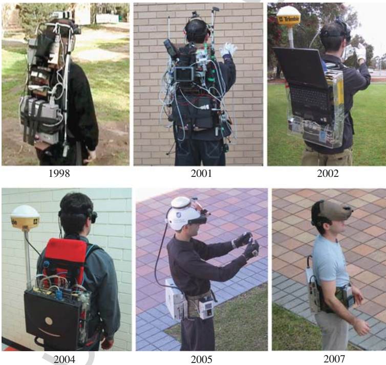
Fig. 11.2 1998–2007: 10 years of Tinmith outdoor wearable computers
