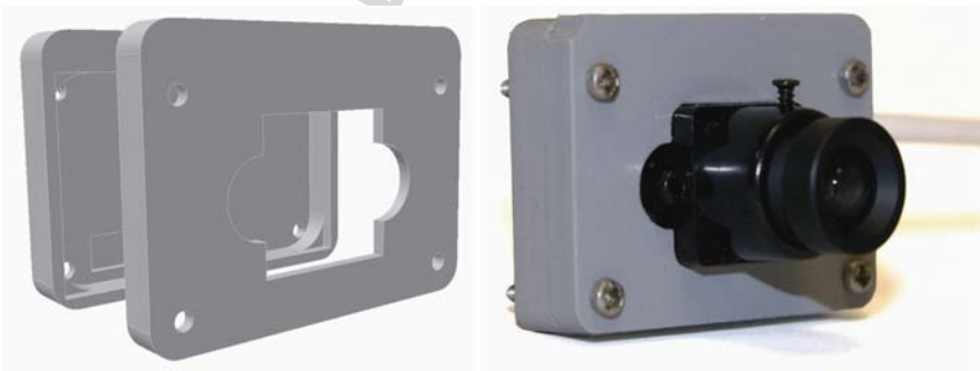
Fig. 11.8 A CAD model of a camera enclosure and the CNC-machined final product
