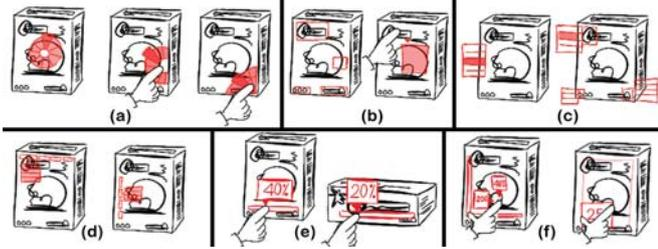
**Fig. 4:** User Interface controls. (a) Dynamic Menu. (b) Mapped Menu. (c) Off-object Menu. (d) Dropdown Menu. (e) One-dimensional slider bar. (f) Two-dimensional slider bar.
