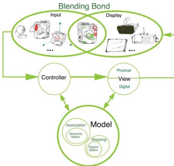
**Fig. 2:** Blended UI Controls Model, a blended adaptation of the original Model-View-Controller by Krasner and Pope [16]
